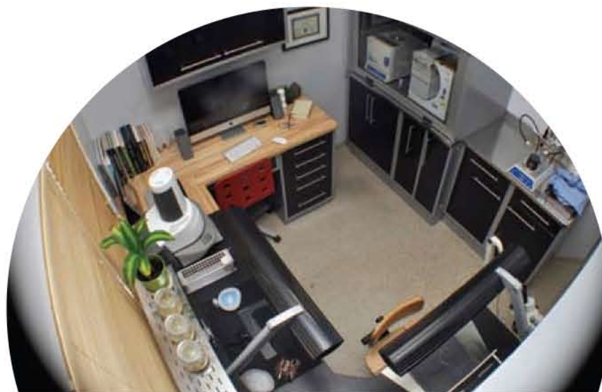
A shot from above the metal/waxing area shows how space is maximized to allow waxing, metal finishing, casting, burnout, pressing, manual milling and even a work area and computer all in this small space. Note that the burnout oven and vacuum casting machines are enclosed in cabinets to eliminate fumes.
