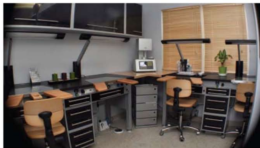
A shot from above the metal/waxing area shows how space is maximized to allow waxing, metal finishing, casting, burnout, pressing, manual milling and even a work area and computer all in this small space. Note that the burnout oven and vacuum casting machines are enclosed in cabinets to eliminate fumes.
