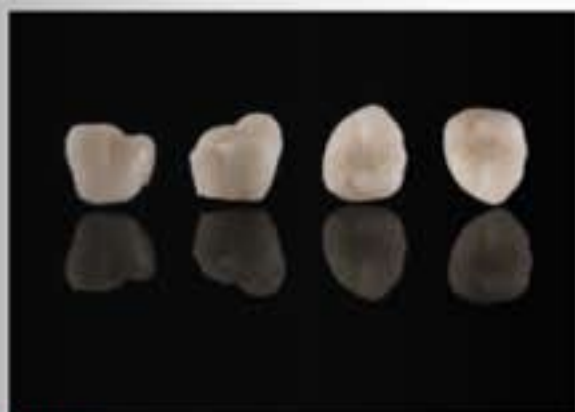
Fig. J The pressing is inspected after devesting.
